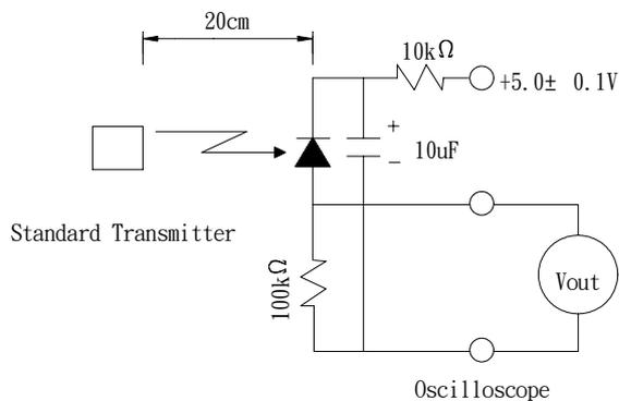
Fig.-3 Measuring System
