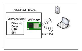
Nano WiReach makes adding WiFi connectivity to embedded devices a breeze. It does not require any kind of WiFi driver development on the host CPU, and its multiple interface (UART, SPI, RMII and USB) minimize the need to redesign the host device hardware.
